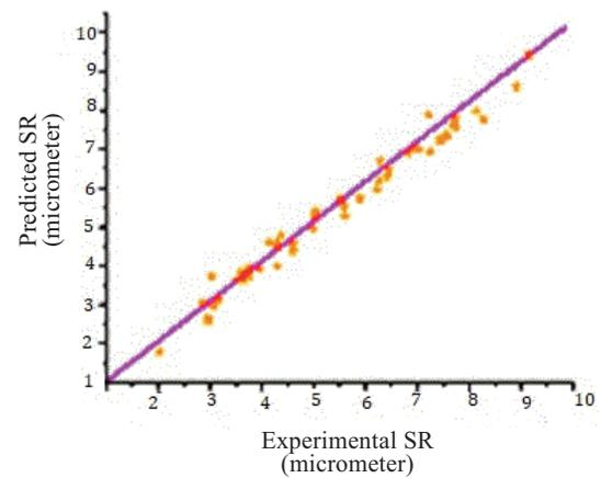
**Fig. 4.** The actual and predicted values of surface irregularity by 3-6-1 neural system.
