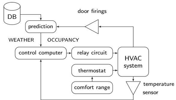
Fig. 1. Pulse-width modulation control of a HVAC system.
