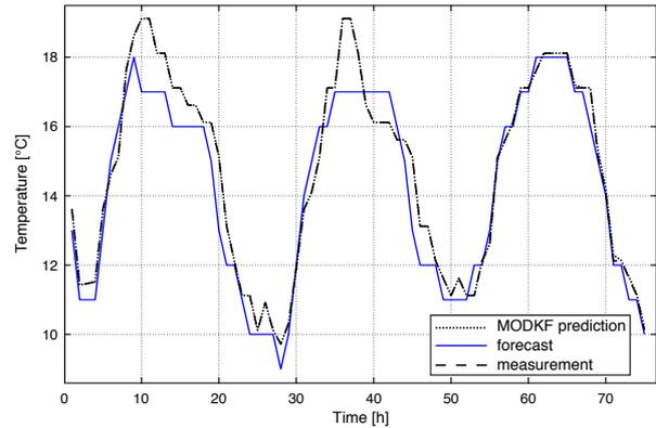
Fig. 4. Temperature estimation based on MODKF.
