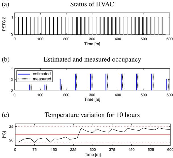
**Fig. 7.** Performance of the PSTC 2 algorithm for a normal day.
