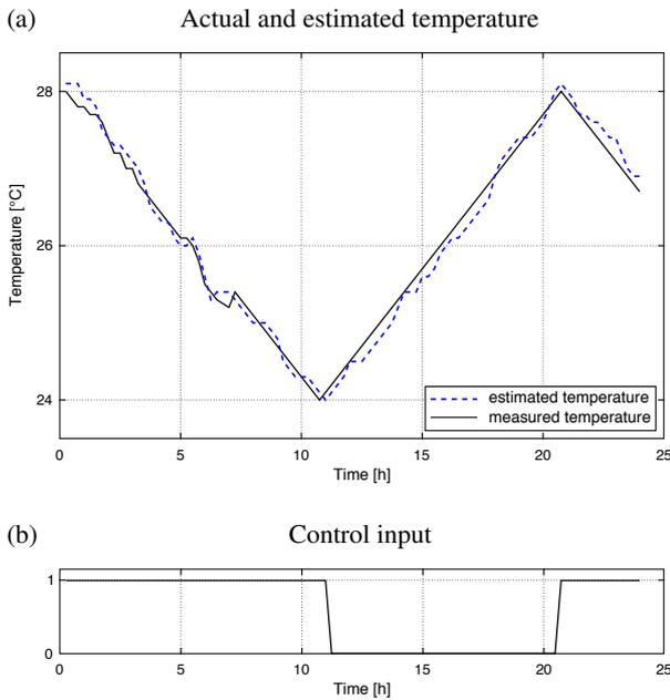
Fig. 2. Room temperature response to the HVAC.
