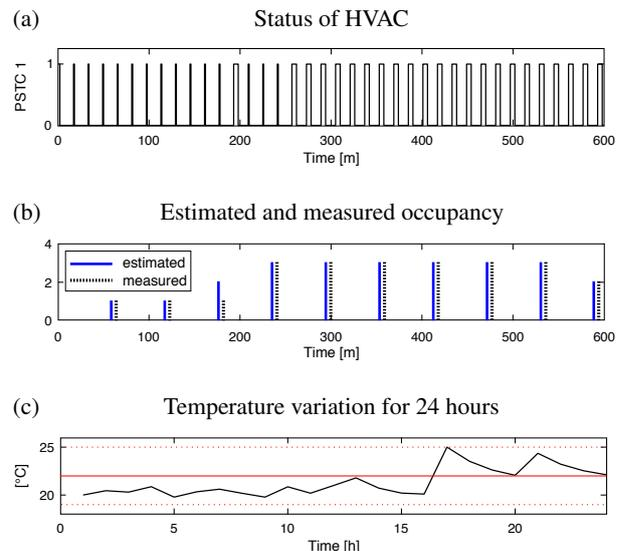
Fig. 6. Performance of the PSTC 1 algorithm for a normal day.
