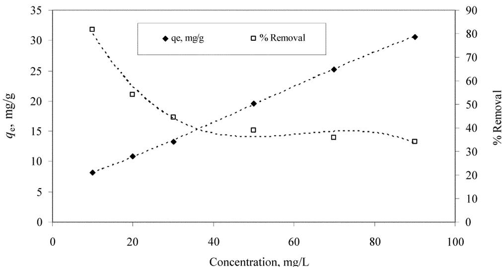
Fig. 4. Effect of the initial dye concentration on dye adsorption.
