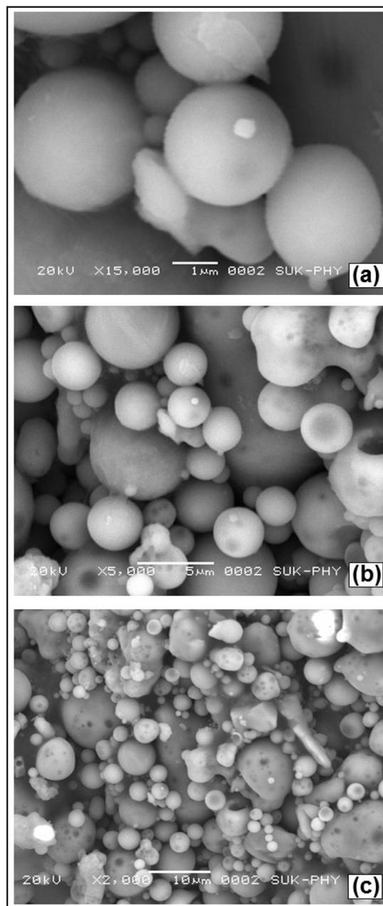
Fig. 1. SEM micrographs of the fly ash.
