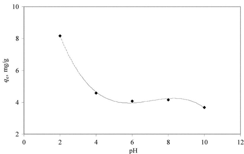
Fig. 3. Effect of the solution pH on reactive blue dye adsorption.
