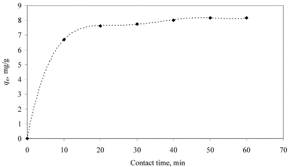
**Fig. 5.** Effect of the adsorbate–adsorbent contact time on reactive blue dye adsorption.
