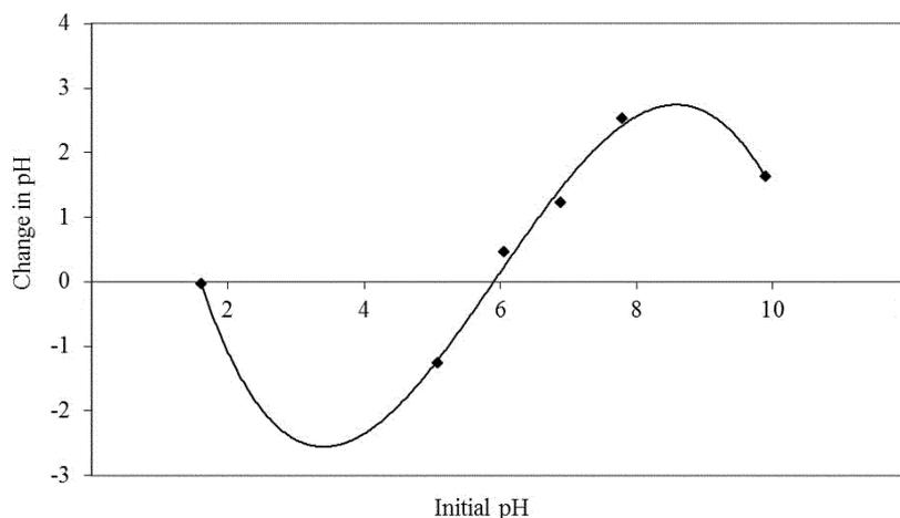
Fig. 2. Change in solution pH versus initial pH.
