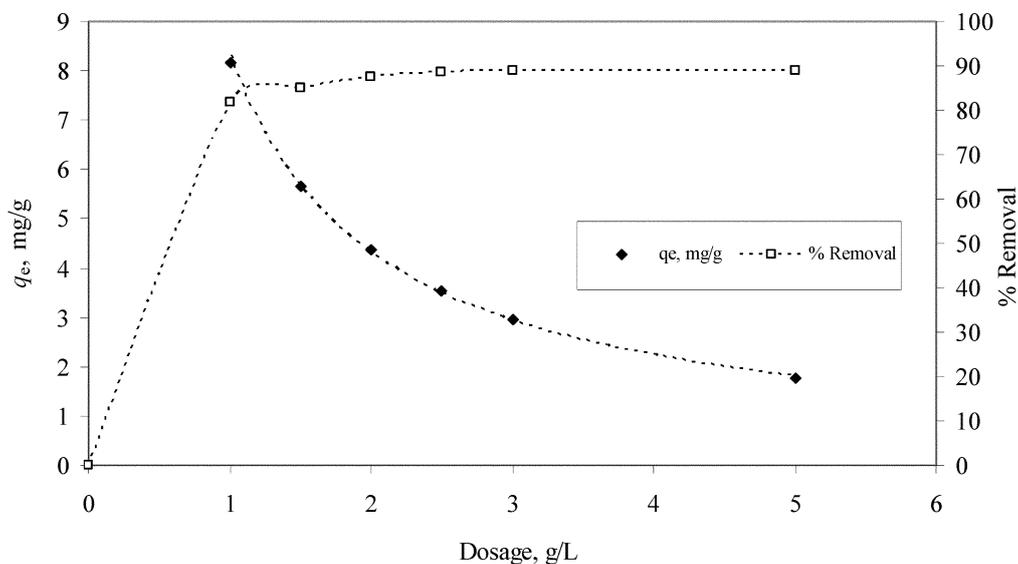
Fig. 6. Effect of the fly ash dosage on reactive blue dye adsorption.
