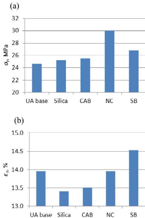
**Fig. 2.** The effect of the additive on the elongation (a) and tensile strength (b) at the yield point.
