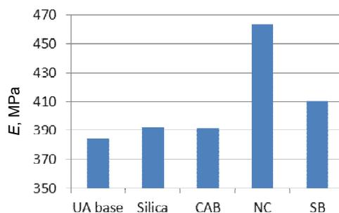
Fig. 1. The effect of the additive on the modulus of elasticity of the film.
