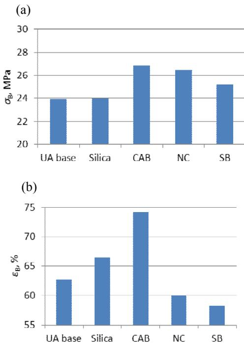
**Fig. 3.** The effect of the additive on the elongation (a) and tensile strength (b) at the break point.
