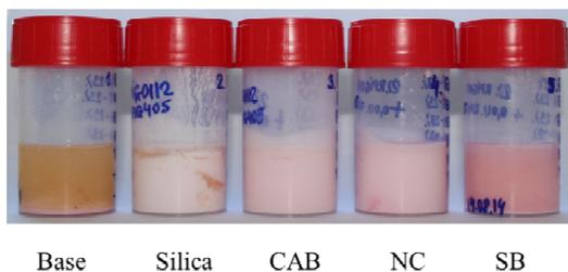
**Fig. 4.** Additive effect on pigment stability of pigmented suspensions after 4 weeks at 50 °C.
