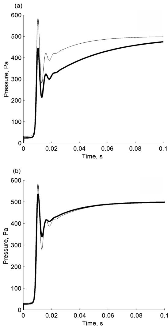
**Fig. 4.** Simulated pressure waveforms: (a) for baseline conditions (thin) and for increased R1 (bold), (b) for baseline conditions (thin) and for increased R2 (bold).
