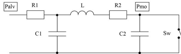
**Fig. 3.** Electrical model for interrupter measurements consisting of two resistors (R), an inductor (L), and two capacitors (C).  $P_{\text{mo}}$  – mouth pressure,  $P_{\text{alv}}$  – alveolar pressure, Sw – interrupter switch.
