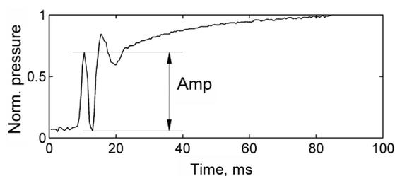
**Fig. 2.** Finding the oscillation amplitude (Amp) as the difference between the first pressure maximum and minimum.
