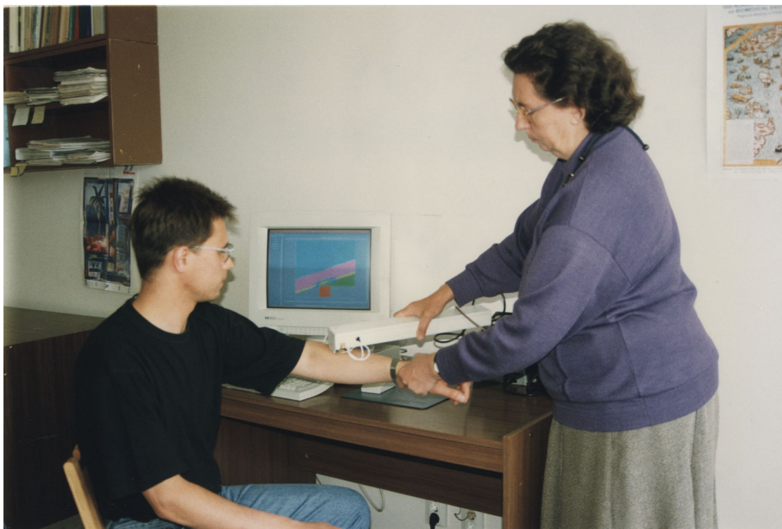
Fig. 2. PhD student Jevgeni Riipulk and Professor Hiie Hinrikus are testing microwave radiometer (1996). Microwave part of the device (two input waveguides, modulator, ferrite isolators, mixer, intermediate frequency amplifier) is located inside the white box.
