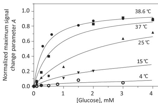
**Fig. 2.** Dependence of the normalized maximum signal change parameter  $A$  on glucose concentration at different temperatures. Measurements were carried out in stirred 0.1 M acetate buffer solution (pH = 5.60),  $[O_2]_{t=0} = 6.6 \text{ mg L}^{-1}$ , final concentration of GOD  $0.036 \text{ IU mL}^{-1}$ .
