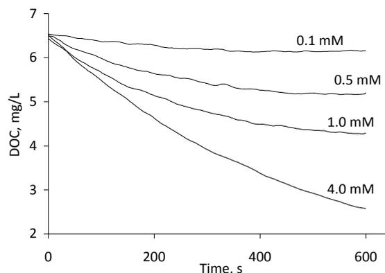
**Fig. 1.** An example of the decrease of dissolved oxygen concentration (DOC) in time at different substrate concentrations. Measurements were carried out with a fibre-optical oxygen sensor in stirred 0.1 M acetate buffer solution (pH = 5.60) at 25°C,  $[O_2]_{t=0} = 6.6$  mg L<sup>-1</sup>, final concentration of GOD 0.036 IU mL<sup>-1</sup> at different glucose concentrations.
