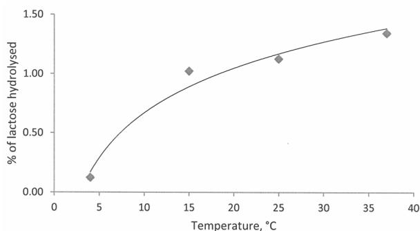
**Fig. 4.** The efficiency of lactose  $\beta$ -GAL-catalysed hydrolysis at different temperatures. Measurements were carried out in stirred 0.1 M acetate buffer solution (pH = 5.60),  $[O_2]_{t=0} = 6.6 \text{ mg L}^{-1}$ , final concentration of GOD  $0.036 \text{ IU mL}^{-1}$  and  $\beta$ -GAL  $3.60 \text{ IU mL}^{-1}$ ,  $[\text{lactose}]_{t=0} = 0.14 \text{ mol L}^{-1}$ .
