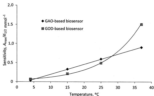
**Fig. 3.** Sensitivity of GOD-based glucose and GAO-based galactose biosensors at different temperatures. Measurements with GOD were carried out in 0.1 M acetate buffer solution (pH = 5.60), final concentration of GOD  $0.036 \text{ IU mL}^{-1}$  and with GAO in 0.1 M phosphate buffer solution (pH = 7.0), final concentration of GAO  $0.036 \text{ IU mL}^{-1}$  under constant stirring;  $[O_2]_{t=0} = 6.6 \text{ mg L}^{-1}$ .
