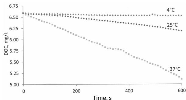
**Fig. 5.** Decrease of dissolved oxygen concentration (DOC) in time at different temperatures in milk-acetate buffer solutions (1 : 1, pH = 6.50) measured with a  $\beta$ -GAL- and GOD-based lactose cascaded biosensing system. Measurements were carried out with a fibre-optical oxygen sensor in a stirred 1 : 1 solution of raw milk and 0.1 M acetate buffer solution (pH = 5.60); final concentration of GOD  $0.036 \text{ IU mL}^{-1}$  and  $\beta$ -GAL  $3.60 \text{ IU mL}^{-1}$ .
