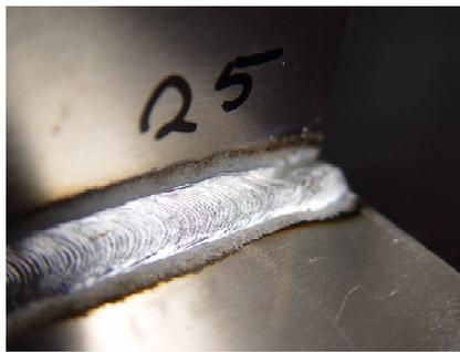
Fig. 2. T-joint, fabricated with welding speed of 12 mm/s;  $U = 14.1$  V,  $I = 143$  A.
