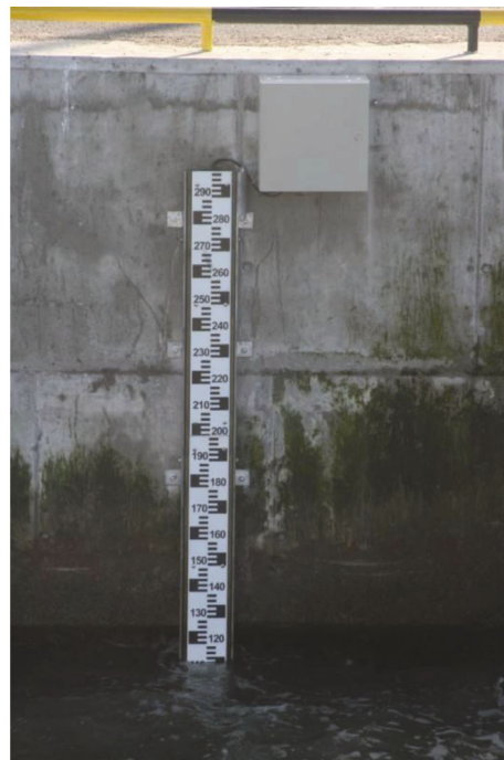
Fig. 2. Typical sea level observation station. The sensors are submerged behind and below the staff gauge and connected by cable to the box of the data handling unit (right above the staff gauge).
