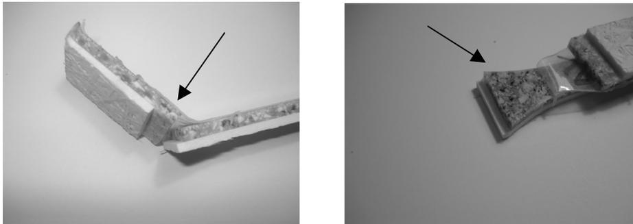
**Fig. 3.** The acrylic material breakdown.
