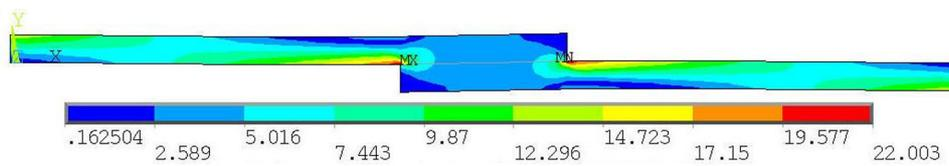
**Fig. 5.** First step of the loading (equivalent stress plot); stresses are given in MPa.
