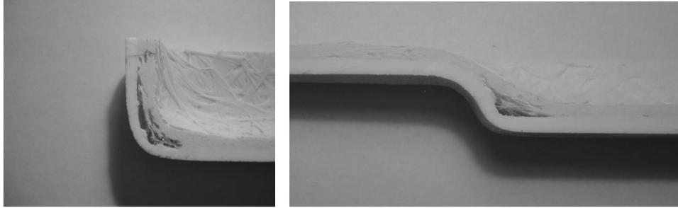
**Fig. 1.** The samples with defective adhesion in the corner (open space between layers).
