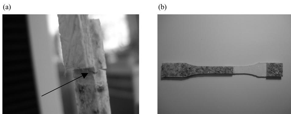
**Fig. 4.** Cracked acrylic material (a) and optimal cut-outs (b).
