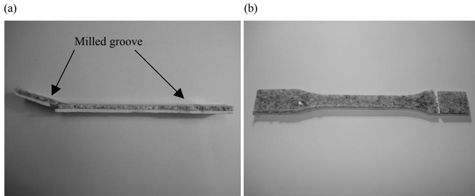
**Fig. 2.** The side view (a) and top view (b) of the test specimen.
