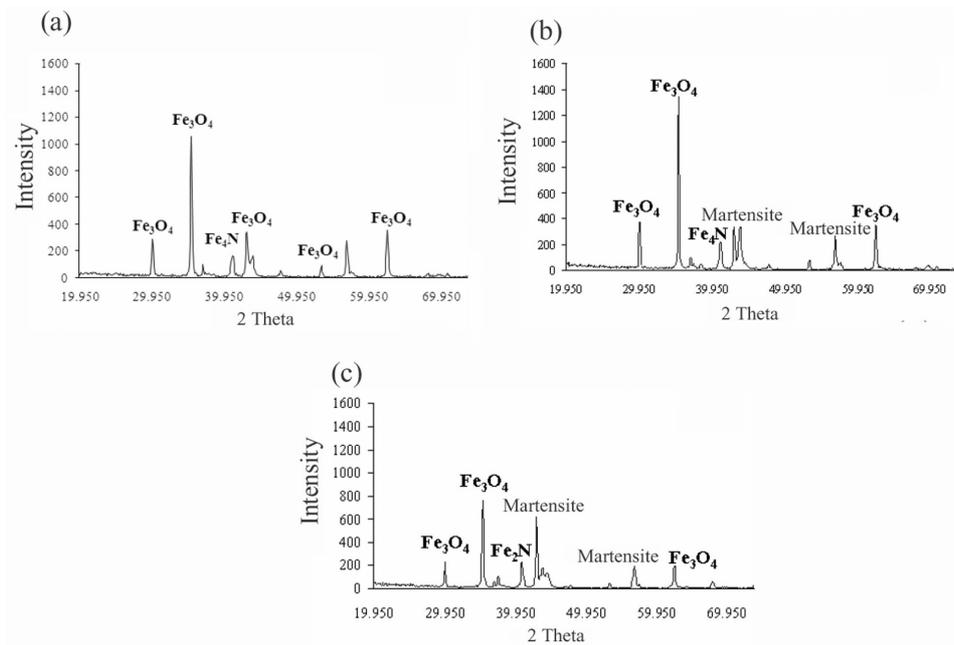
**Fig. 2.** XRD spectra of unworn tool steel 3 specimens: (a) post-oxidation 1, (b) post-oxidation 2, (c) post-oxidation 3.
