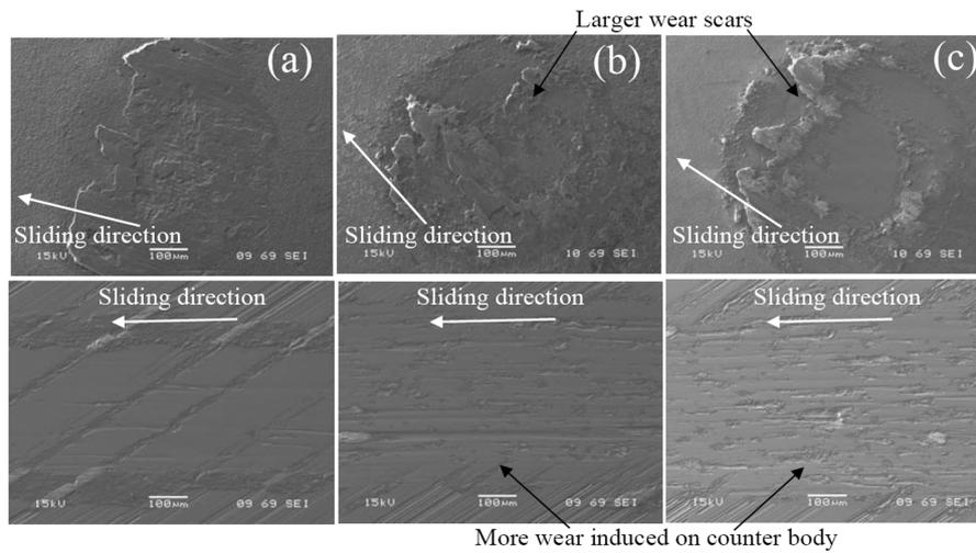
**Fig. 5.** SEM micrographs of wear scars (top-pin, bottom-disc) from room temperature tests: a – tool steel 3, post-oxidation 1; b – tool steel 3, post-oxidation 2; c – tool steel 3, post-oxidation 3.
