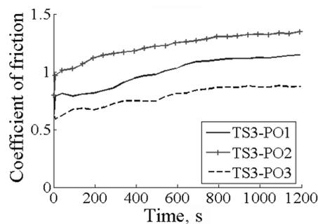
**Fig. 6.** Friction coefficient of tool steel 3, post-oxidations 1, 2 and 3 sliding against the UHSS disc at 400 °C.
