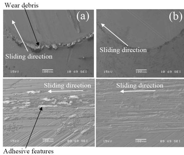
**Fig. 4.** SEM micrographs of wear scars (top-pin, bottom-disc) from room temperature tests: a – tool steel 1, post-oxidation 1; b – tool steel 2, post-oxidation 1.
