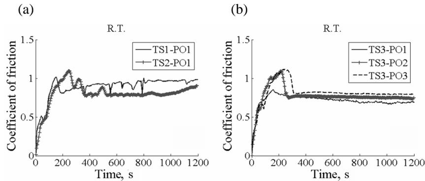
**Fig. 3.** Friction coefficients of tool steel 1 and tool steel 2 with post-oxidation 1 (a) and tool steel 3 (post-oxidations 1, 2 and 3) sliding against UHSS disc at room temperature (b).
