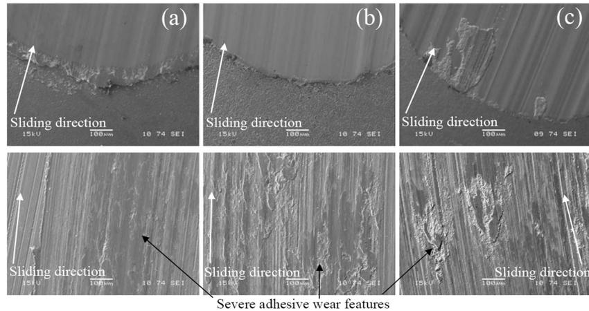
**Fig. 7.** SEM micrographs of wear scars (top-pin, bottom-disc) from tests at 400 °C: a – tool steel 3, post-oxidation 1; b – tool steel 3, post-oxidation 2; c – tool steel 3, post-oxidation 3.
