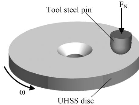
**Fig. 1.** Schematic of the test specimen configuration.
